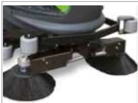
PRE-SWEEP SYSTEM ON CYLINDRICAL MODEL
