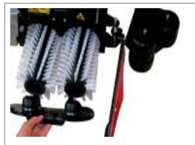
COMBINED SCRUBBING-SWEEPING SYSTEM THAT INCLUDES DEBRIS HOPPER ON CYLINDRICAL
